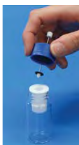
Put in the MonoTrap after sampling. Close the vial and ultrasonicate
