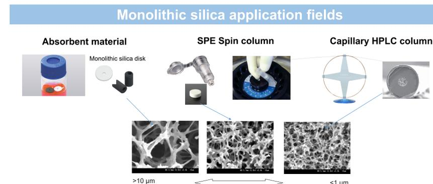
The pores can be sized according to application, resulting in a highly adaptive material for chromatography.
