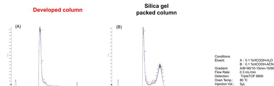
Intact mAb mass analysis (total ion chromatogram) on (A) an developed column, (B) silica packed column.
