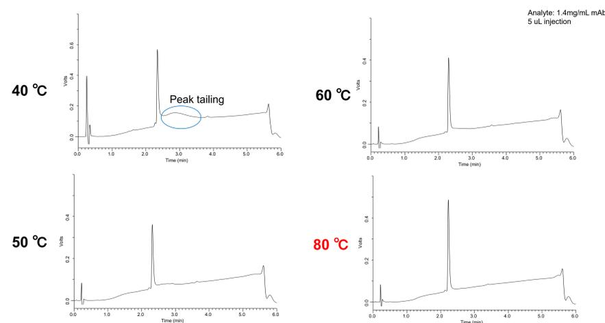
Separation of Intact mAb using a developed monolithic column at different temperatures.
