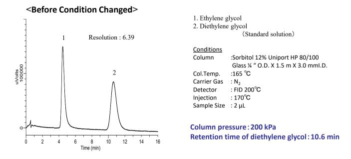
Before changing the conditions, even under column pressure of 200 kPa, the retention time of diethylene glycol was 10 min, exceeding the stipulation of test method, but resolution was within the specifications.
