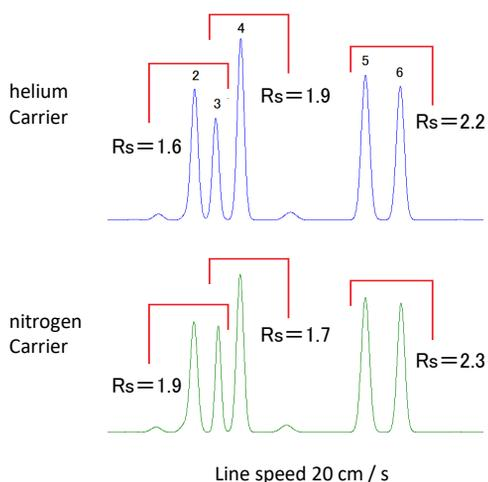
When the carrier gas is changed from helium to nitrogen, it can be seen that the peak resolution after changing the carrier gas visually decreases at linear velocities around 40 cm/s. When changing the carrier gas, compare the degree of peak separation under the analysis conditions in which the linear velocity is set to be gradually decreased as shown below.
