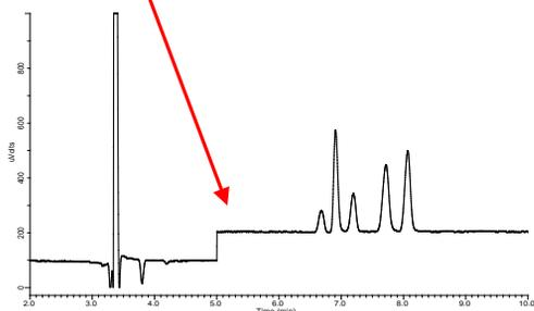
The baseline may be disturbed when the polarity changes, but if it does not overlap with the peak, there is no problem with the analysis.
