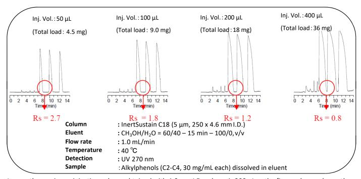
In case the maximum injection volume obtained with 4.6 mm I.D. column is 200  $\mu$ L as the figure shown above, the maximum injection volume of preparative column is estimated as follows. Detail of scaling up is described in LC Technical Note No.134.
