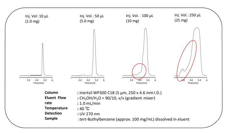
In case the maximum injection volume obtained with 4.6-mm I.D. column is  $100 \mu L$  as the figure shown above, the maximum injection volume of preparative column is estimated as follows. Detail of scaling up is described in LC Technical Note No.134.
