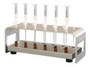
This is a Free fall manifold that can use multifunctional mini column for aflatoxin pretreatment and 4 mL vial as a receptacle.
