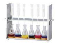
Racks used to extract solid phase by free fall such as InertSep K-solute. Adjusting the height of the stand allows the user to select and set the size and position of the receiver.
